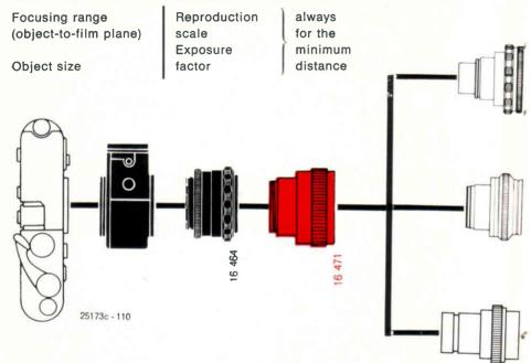
Black: data and adapters for normal focusing range Coloured: data and adapters required for the close-up and the macro range respectively (All values are rounded off).
