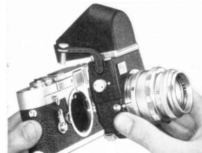
The VISOFLEX III mirror reflex attachment with quick-change bayonet mount can be used on any LEICA®-M body. It can be changed as a complete unit like any LEICA lens. It is simple and easy to operate. But since the VISO-FLEX offers an unusual number of possibilities. we would suggest that you study these brief instructions at leisure. It will give you much good advice and thus further increase the pleasure of using your LEICA equipment.
